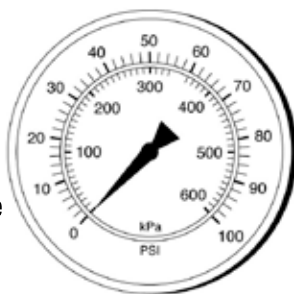
Typical Pressure Gauge
