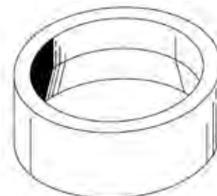
Typical One-Piece Ring Compressor
