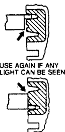
1U6431 KEYSTONE PISTON RING GROOVE GAUGE GROUP
