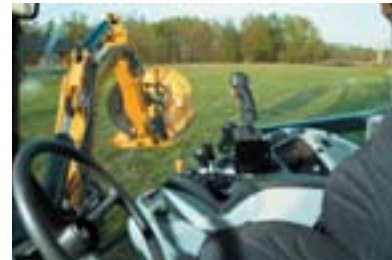
A single, primary grade, electronic joystick linked to an electronic proportional four-way hydraulic spool valve, provides simultaneous control of multiple boom functions.
