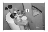
At the top of the stretch rolls, 4 magnets rotate below the stretch sensors (1=B109).
