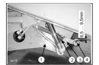
The rod (4) is pressed down by the belt of the wrapping table when a bale is on the wrapping table. This motion actuates the actual value switch (2=Z92).
