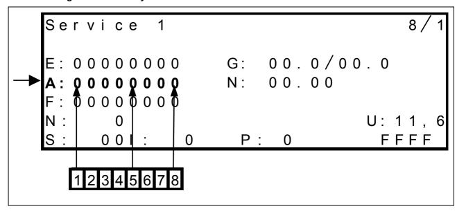
Eight numeric characters are available for output diagnosis in line "A", each of them being assigned to one solenoid valve.
