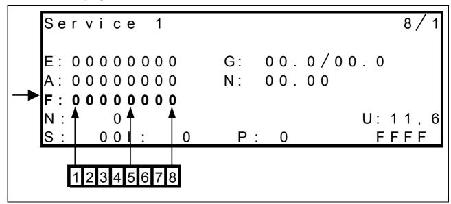
Eight numeric characters are available for error display in line "F", each of them being assigned to one error.
