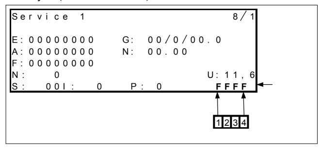
Four numeric characters are available for key testing in line (1) shown above.
