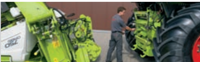
Ease of access to knife drum
