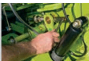
Mechanical shear bar adjustment
