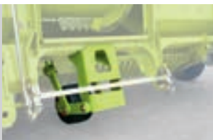
Support wheel for optimal ground-contour following
