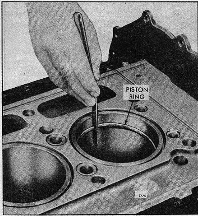
FIG. 26 - Measuring Piston Ring Gap
