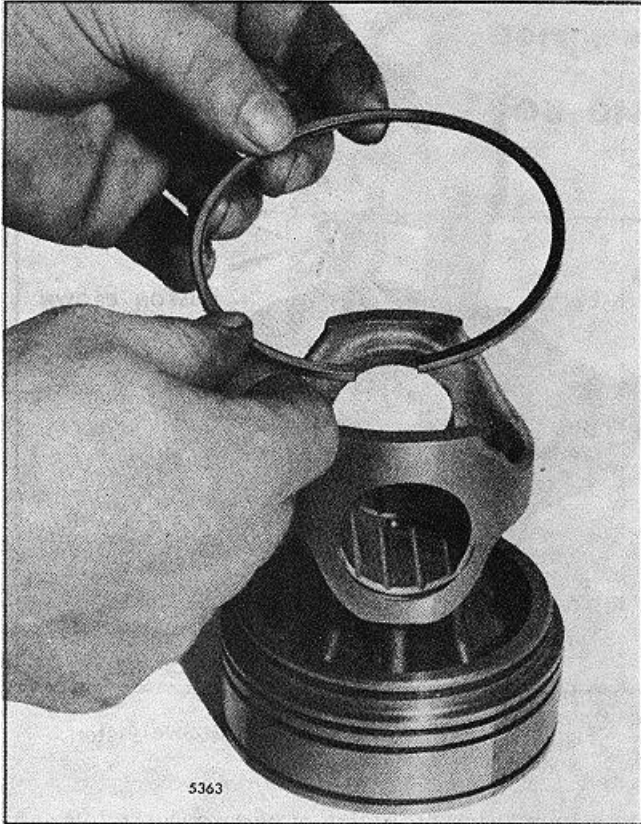
FIG. 18 - Installing Seal Ring
