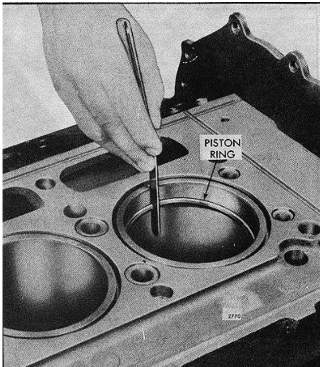
FIG. 9 Measuring Piston Ring Gap
