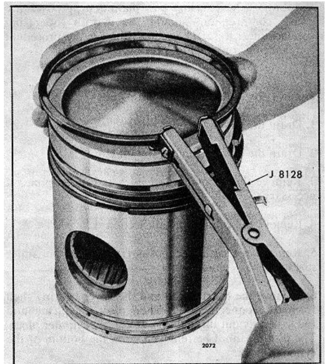
FIG. 2 Removing or installing Piston Rings
