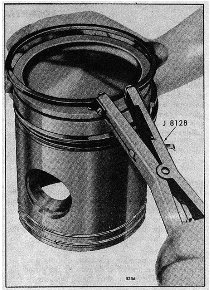
FIG. 16 - Removing or Installing Piston Rings
