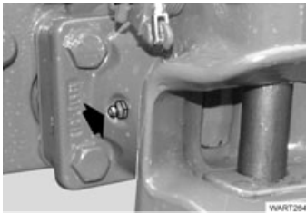
Automatic trailer hitch with cylinder-type bolt.
