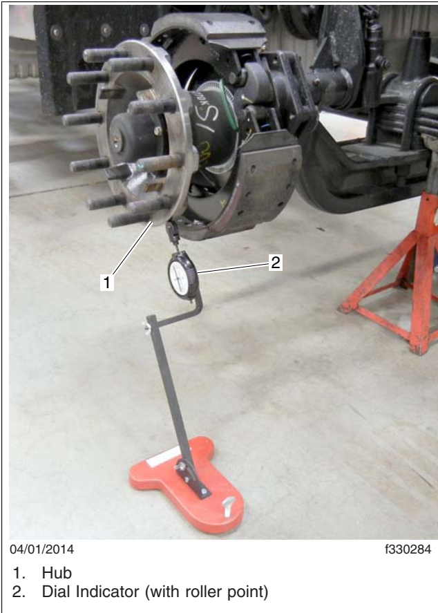
Fig. 2, Setup to Measure Radial Runout
