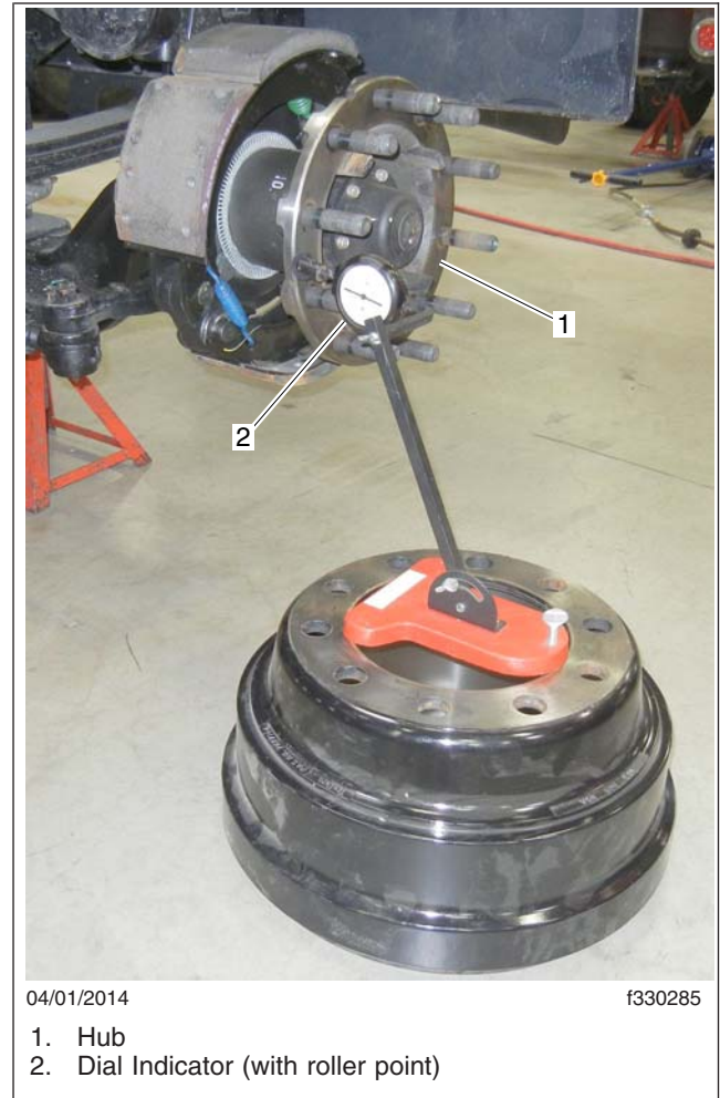
Fig. 1, Setup to Measure Lateral Runout
