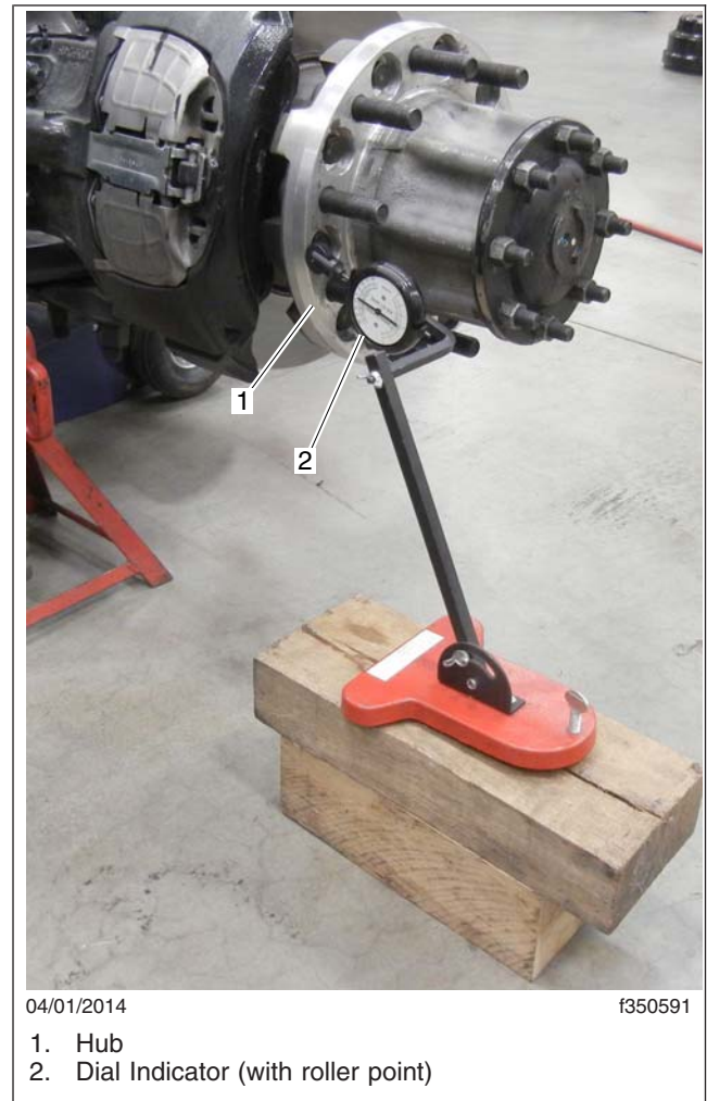
Fig. 1, Setup to Measure Lateral Runout
