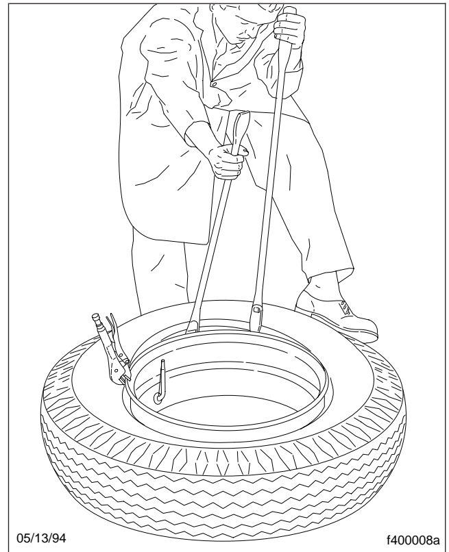
Fig. 6, Working the Upper Bead into the Rim
