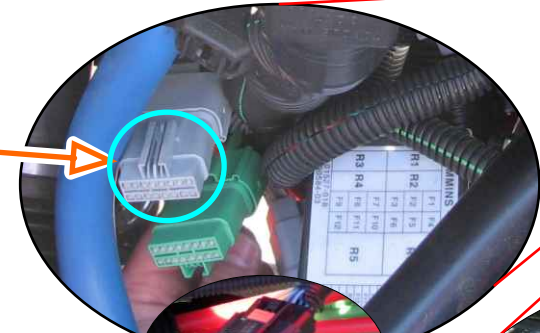
Transmission Interfaces. (Grey Plug) (Plugs may also be frame located (Module , 34C)
