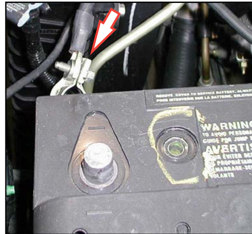
Illustration BA-20 Negative (black) Cable Disconnected and Tucked Away
