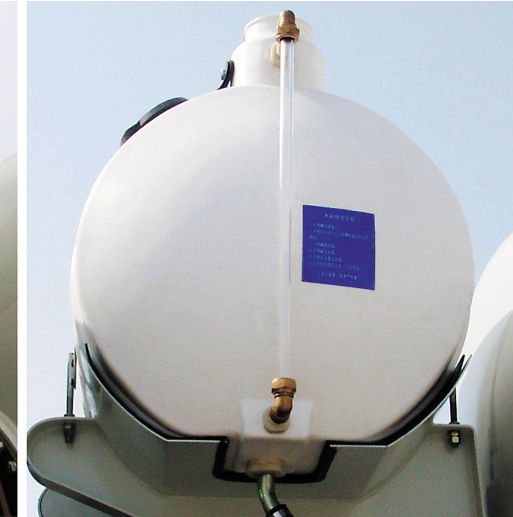
Water pump supply water tank
